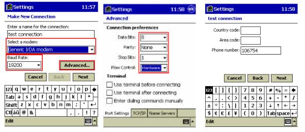
Figure 1. Select a modem and check the Baud Rate (When using HSCSD it is recommended to use I e 57400). After that tap Advanced... Figure 2. Check Connection preferences. Especially that the Flow Control selected is HW. Tap OK on upper right corner and then tap Next Figure 3. Type in the ISP's phone number (typically in GPRS Connection the ph. number is \*99#, please check from your GSM operator) and then tap Next.
